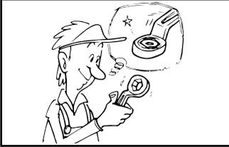
13. Tighten further if any screws, bolts and nuts are loose.
